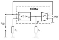
Fig. 6. Positive immitance converter built from CCIITA
