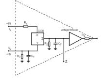
Fig. 2. Block realization of transimpedance amplifier CFA
