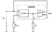
Fig. 5. Immitance inverter built from CCIITA
