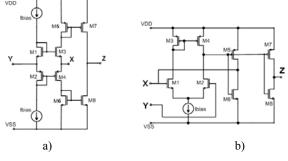
Fig. 9. Internal topology of current conveyor CCII+ a) based on current mirrors b) based on opamp structure
